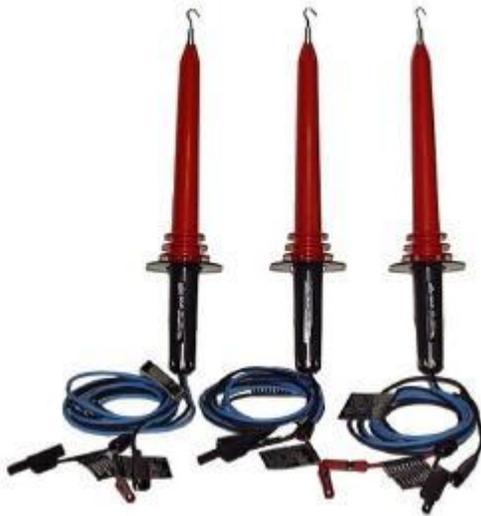
Each probe comes with a hook attachment to facilitate hands-free measurement and long term monitoring of 5KV lines. Each probe has a ground clamp, a neutral connector and a reduced voltage connector. The connectors are safety banana plugs. Each lead is labeled to advise how to use it.
