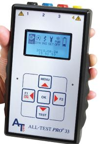
AT33IND<sup>™</sup>,which is used for de-energized Motor Circuit Analysis (MCA<sup>™</sup>), is specifically designed for troubleshooting motors and commissioning new and rebuilt motors before installation. The AT33IND<sup>™</sup> enables the operator to identify motor conditions that include winding contamination, stator and rotor unbalance, changes in rotor and stator condition, resistance in windings, contamination, and insulation to ground issues.
