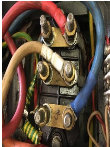
Supply leads touching conductive paths in multiple areas. Red delta link short to earth, too
