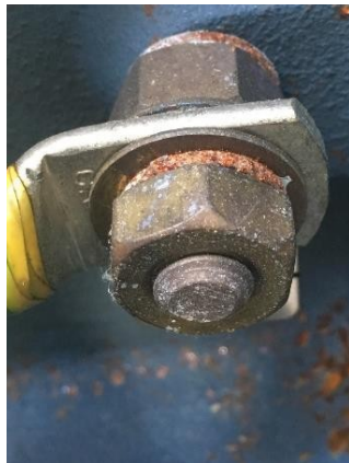
Moisture Ingress, Red Supply Overcrimped
