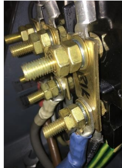
Supply, Delta Links and Motor lugs all together
