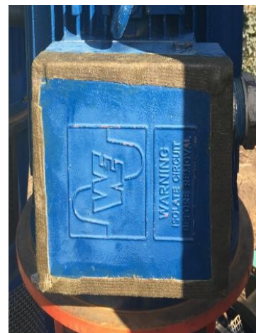
Terminal Box gasket failed
